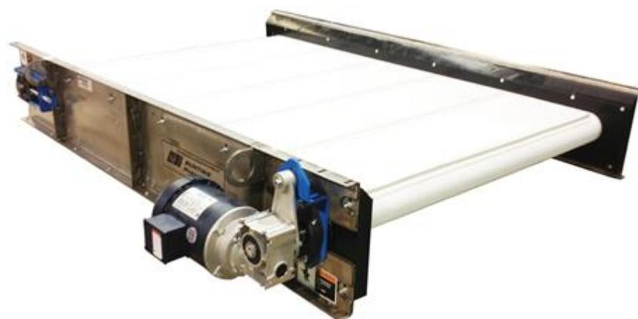
The HISC Magnetic Pulley is 100mm (4") in diameter and up to 1200mm (60") in width. Each unit operates with a thin urethane belts, ensuring that the highest possible gauss intensity is generated on the belt surface. The belts run at between 15 and 60 metres per minute, depending on the application, with speeds being adjusted via an inverter. Positioned under the extremely strong discharge Magnetic Pulleys are adjustable splitters chutes for the separated streams of material.
